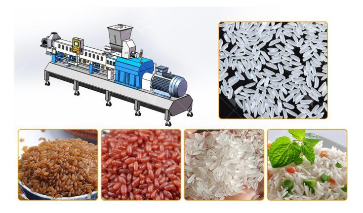
?3?The line can use rice, millet, black rice and buckwheat as the main raw materials. Then it can be treated with vitamins, proteins and mineral substances. After the process of extrusion, steaming and forming, it can make fortified rice, golden rice, buckwheat rice, etc. The steaming method is the same as that of natural rice. Cooking is the same as natural rice, or even easier and more convenient.
