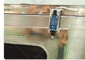
5. The observation window is equipped with a travel switch to prevent microwave leakage and improve safety.
